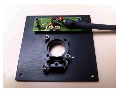
Fasten the XLR chassis to the from plate with the 3 M3 nuts.
